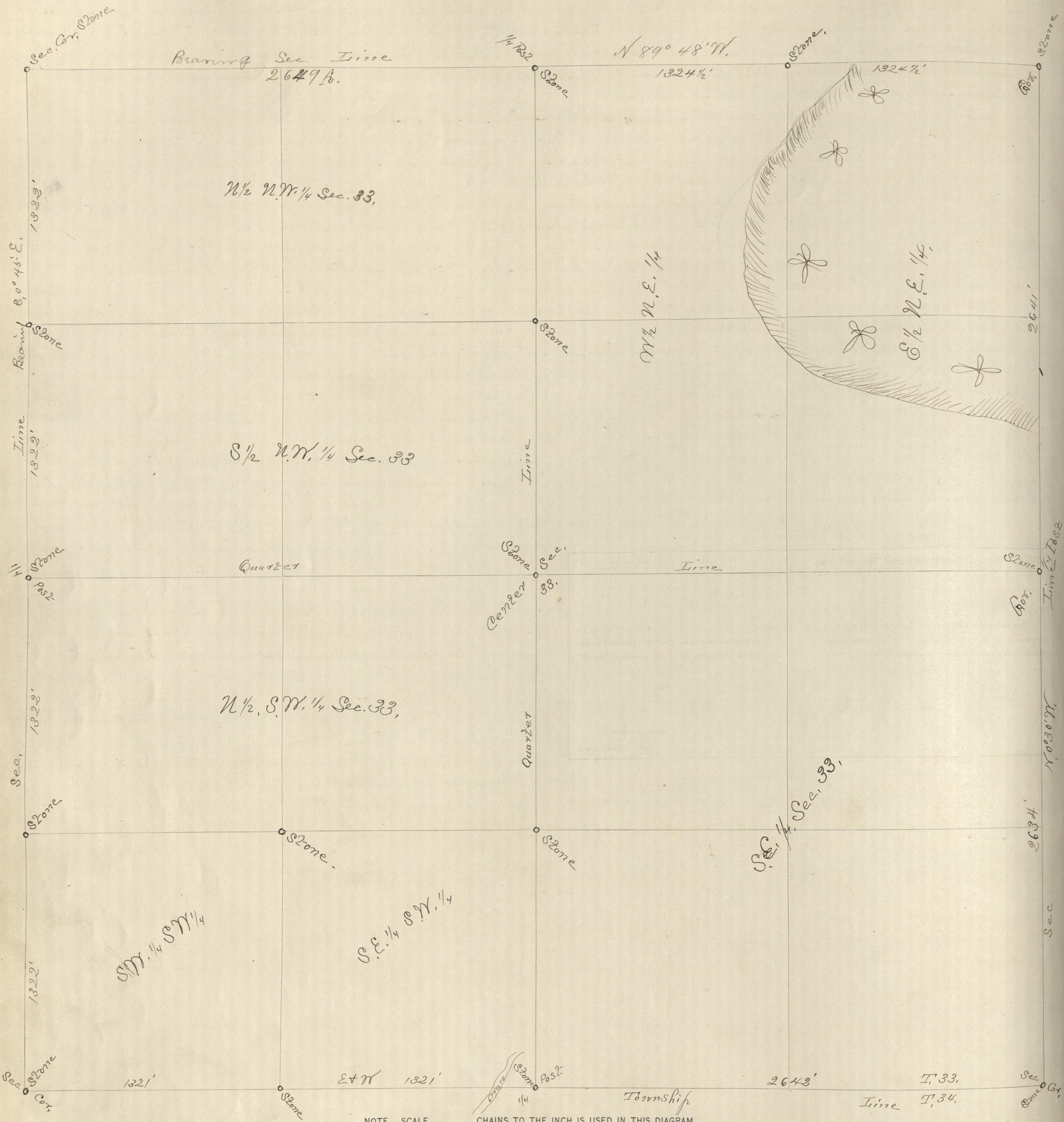
This diagram to be used in platting either one, four or sixteen sections. When used for one section only, scale No. 1 applies; for four sections, scale No. 2; and for sixteen sections, scale No. 3.
