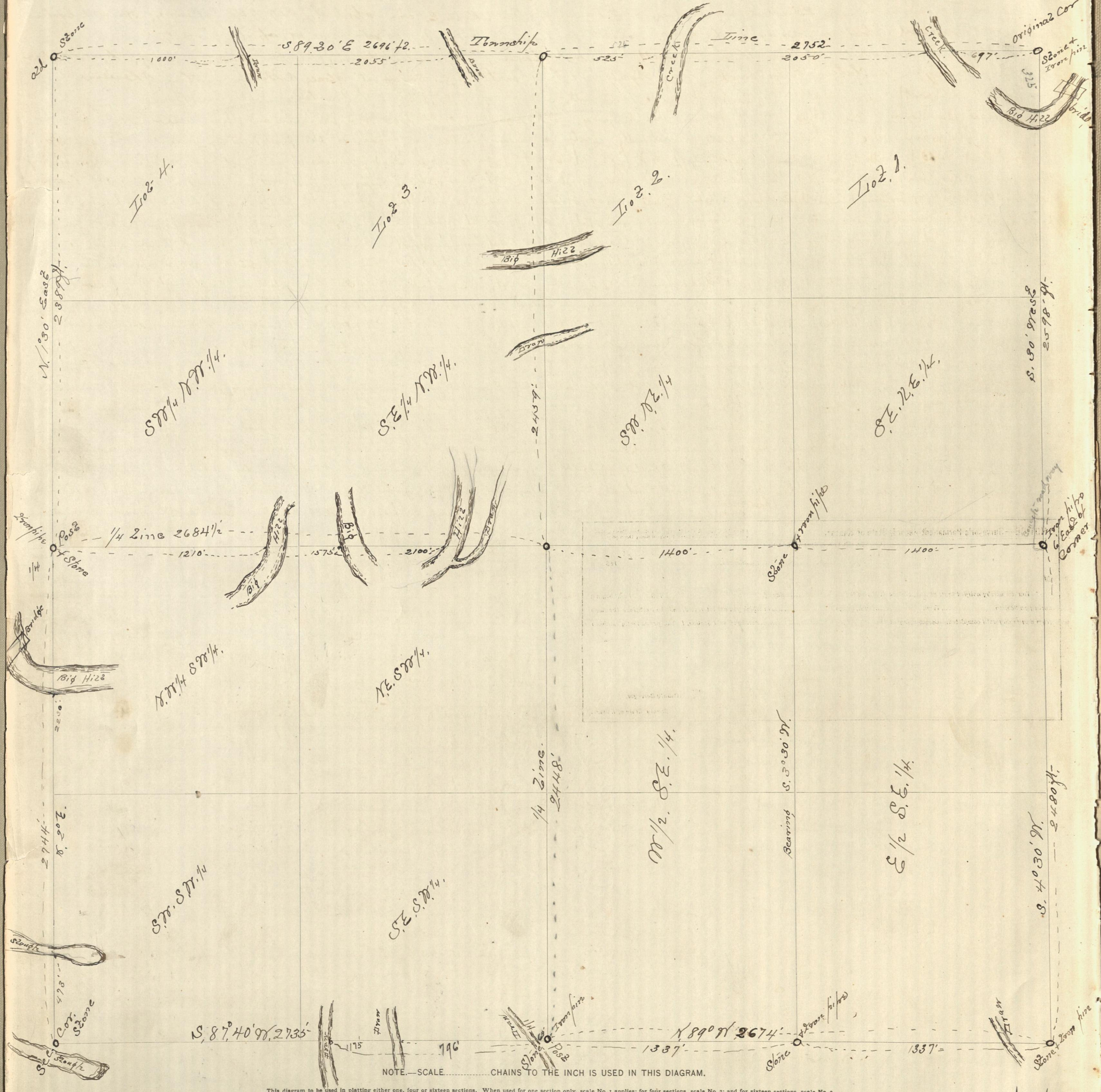
This diagram to be used in platting either one, four or sixteen sections. When used for one section only, scale No. 1 applies; for four sections, scale No. 2; and for sixteen sections, scale No. 3.
